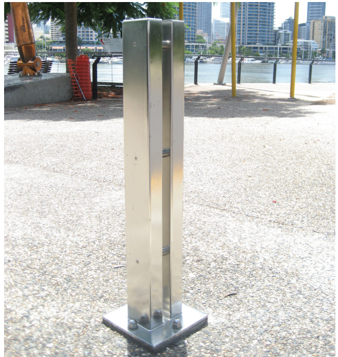
Electropolished stainless steel grade 316 in perfect condition after seven years of exposure in a marine environment.
